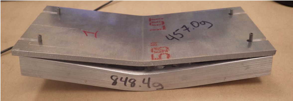
Figure 6. Post-test photo of sample 1 showing permanent bending of the top panel and Tri-comb™ structure.
